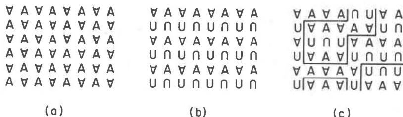
Fig. 36. Schematic diagrams of the pigeonite structure projected down [001] (after Morimoto, 1974). (a) C-centered lattice of high C2/c pigeonite. A and V represent symmetrically identical chains. (b) Primitive lattice of low P2_1/c pigeonite. The A chains are represented by A and V and the B chains by U and N. (c) Domain structure of low pigeonite. Note shift of (a + b)/2 along domain boundaries.
