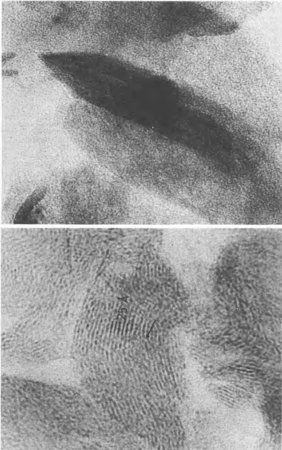
Fig. 2. Electron micrograph of a thin section of (a) dodecylammonium-buserite showing 25 Å spacing and dislocation (arrowed) and (b) Ca-buserite showing 7 Å spacing.
