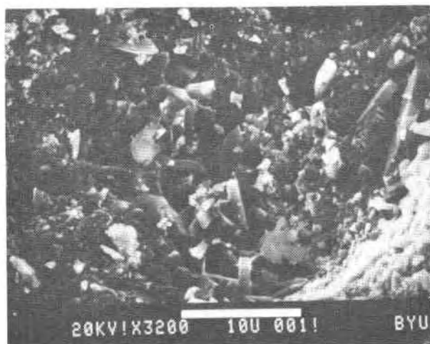
Fig. 1. SEM photomicrograph of synthetic zinc staurolite crystals. Length of scale bar represents 10 microns. Angles measured on this and other SEM photos suggest that the large crystal faces are (010), modified by (110), (201), and (201), with crystals elongated on c.
