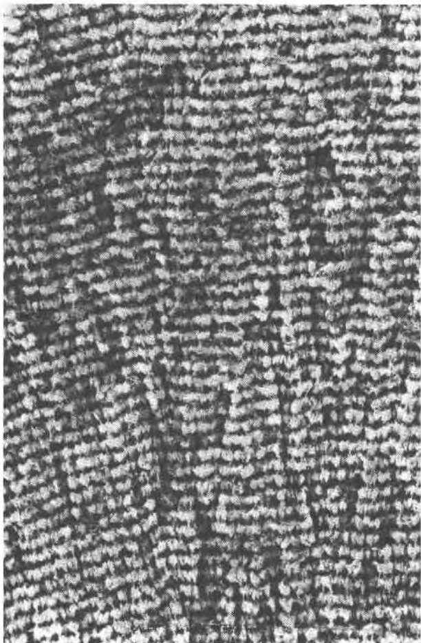
Fig. 1. SEM photograph of differentially etched oscillatory zoning in chalcedony. The light bands are approximately 1 micron wide.
