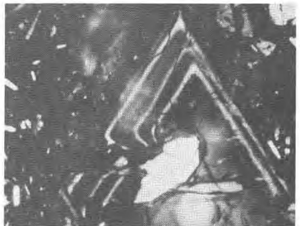
Fig. 2. Photomicrograph of the plagioclase crystal of Figure 1, showing zones. Crossed Nicols.
