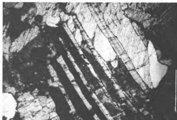
Fig. 6. Photomicrograph of sample 2345D from Mount Riiser-Larsen, Enderby Land, containing inverted pigeonite. Coarse lamellae in diagonal position, which extinguish simultaneously, are clinopyroxene. These lamellae cut grain boundaries of orthopyroxene, which are present in different optical orientations (light, dark gray, and black). White, featureless grains are quartz. Crossed nicols. Length of bar 1 mm.
