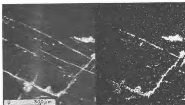
Fig. 3. SEM micrographs of breunnerite with dolomite filling cleavage cracks (left) and Ca distribution (right).
