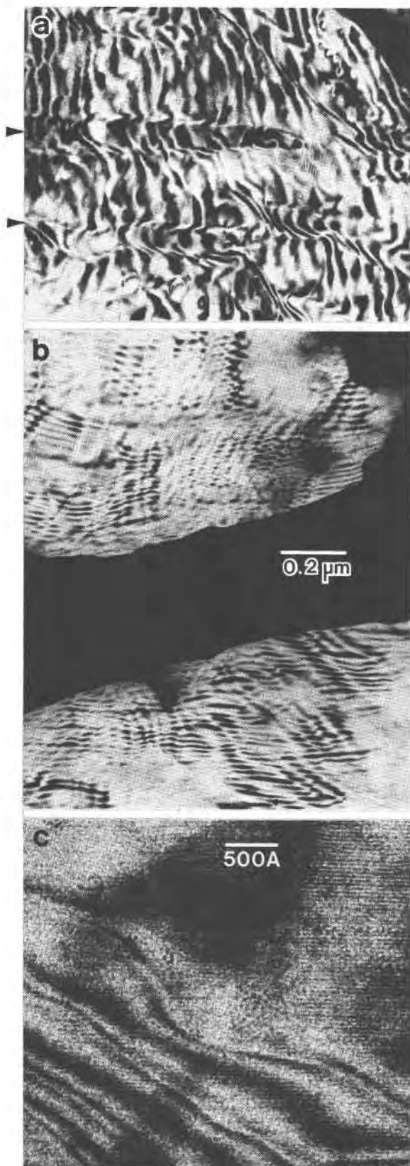
Fig. 5. a. Moiré fringes from turbostratic stacking. The arrows indicate two talc exsolution lamellae (horizontal). b. Two-dimensional moiré pattern. c. Two sets of moiré fringes. The very fine horizontal set of fringes is from a 30^\circ twin, and the coarse, irregular fringes are from turbostratic stacking. The scale in a is the same as in b.
