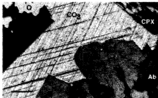
Fig. 5. Photomicrograph showing the relationship of interstitial calcite ( CO_3 ), quartz (Q), albite (Ab), and high-Ca pyroxene (CPX) in the trondhjemite. Transmitted polarized light. Crossed nicols, scale bar = 250 \mu m .
