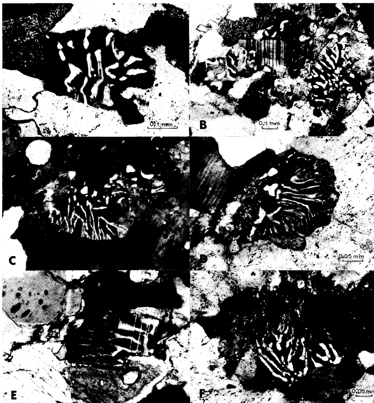
Fig. 1. (A) Myrmekite from the pelitic schist-gneiss unit, surrounded by K-feldspar and biotite. Twinning visible within myrmekitic plagioclase. (B) Myrmekitic plagioclase crystals in pelitic schist-gneiss unit. (C-D) Bulbous myrmekite invading K-feldspar. Micaceous quartzite unit. (E) Dendritic myrmekite showing twinning; in contact with hornblende and K-feldspar. Calc-silicate gneiss unit. (F) Myrmekite surrounded by K-feldspar. Calc-silicate gneiss unit.
