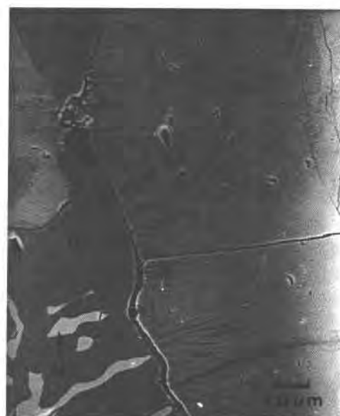
Fig. 2. Secondary electron image of fayalite and pyroxene grains from Hebei. Laihunite grew from the grain edges of fayalite into fayalite. Magnetite appears within the grain of pyroxene.
