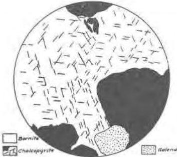
Fig 3—Showing the triangular pattern produced by the nearly equal development of the "intergrowth" in 3 directions.
