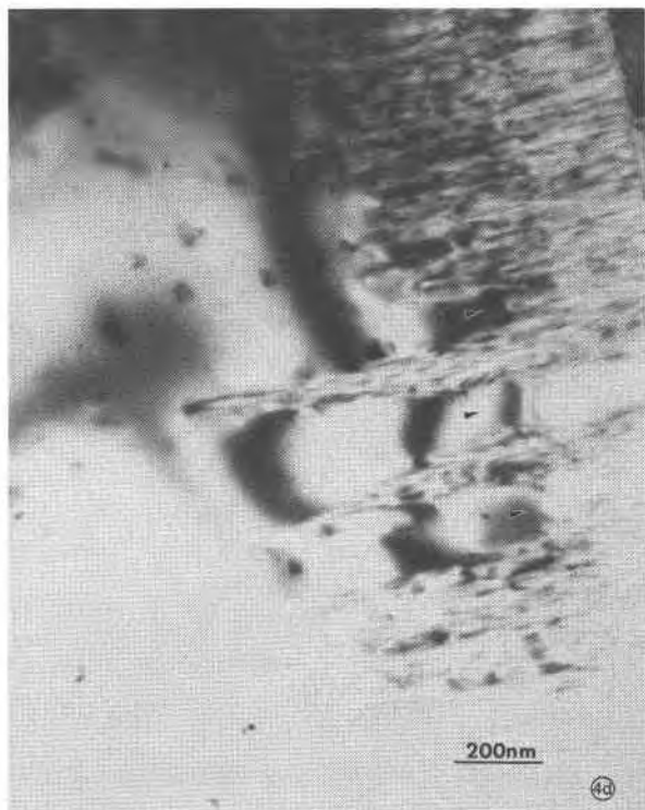
Fig. 4c. Modulated microstructure in lamellar domains of aragonite. Homogeneous interlamellar material is calcite.
