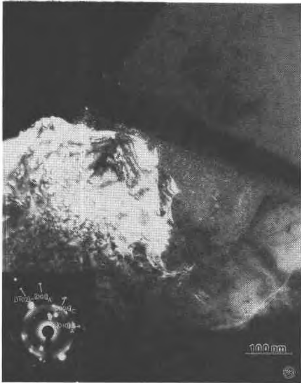
Fig. 7. (a) Darkfield photomicrograph of aragonite plus calcite. Objective aperture is centered on the aragonite (011) reflection. Aragonite appears bright, calcite dark. Note lime rings begin to appear in the SAD and scattered spots in the image signal the onset of decomposition within calcite. (b) Lime rings coarsen and aragonite reflections disappear in the SAD. Lime spots increase in the image. (c) Calcite reflections disappear in the SAD and transformation to lime is ubiquitous in the image. Note widening of the fracture.
