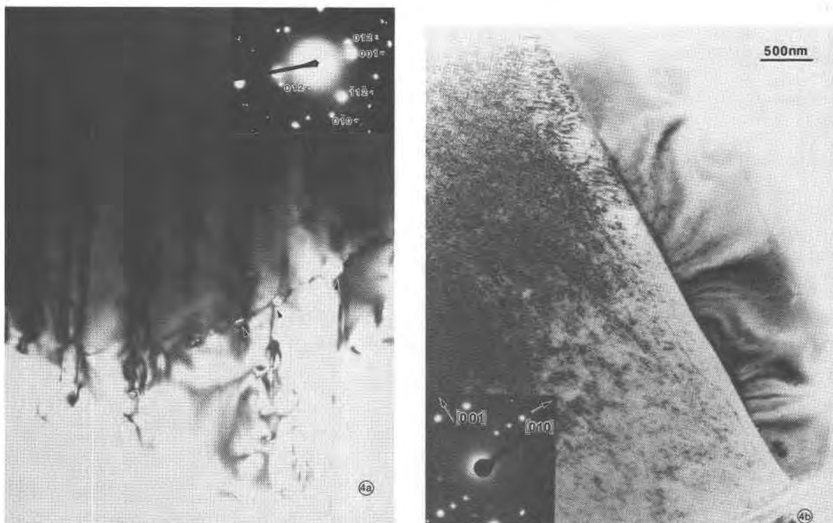
Fig. 4. (a) Calcite nuclei at the intersection of {110} twins and a dislocation in aragonite (arrowed). Dual phase diffraction pattern is inset. (b) Aragonite (right)-calcite (left) grain boundary oriented parallel to (010) in aragonite. Mottled contrast in calcite is due to radiation damage. Note microfracture in the lower right corner.
