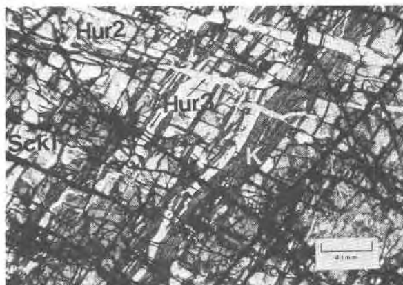
Fig. 8. Photomicrograph of massive, yellow sicklerite (sck1) and minor pale green hureaulite II (hur2) cut by veinlets of yellowish-green phase 'K' (K) and then by veinlets of colorless hureaulite III (hur3). Plain light.
