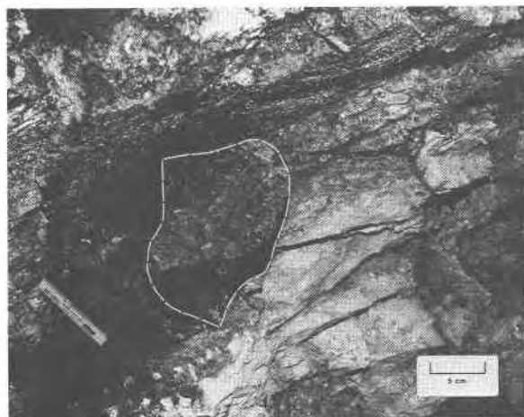
Fig. 3. Photograph of a lithiophilite crystal embedded in pegmatite host rock in the old underground workings of the Stewart Lithia mine. The outline of the crystal has been highlighted with a dashed white line.
