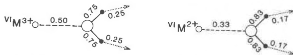
Fig. 17. Bond-valence structure of H 2 O bonded to [6]-coordinate divalent and trivalent cations.
