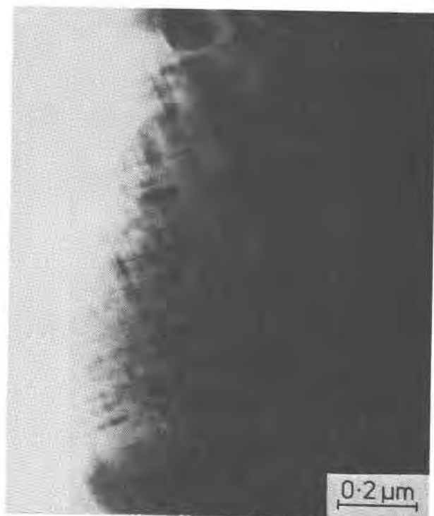
Fig. 3. Typical cross-hatched twinning texture in cristobalite (CR-1). Similar textures were observed in grains from TRIV and TR-G3. Bright field image.
