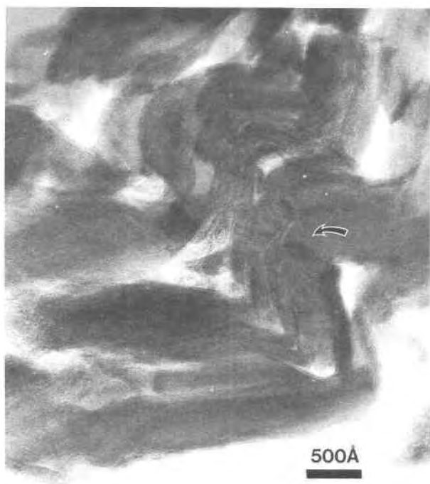
Fig. 3. HRTEM image of Cornwall tochilinite microtomed normal to the cylinder axis, showing en echelon texture. Arrow indicates region where the lattice fringes of the characteristic 10.8-Å spacing of tochilinite are visible.
