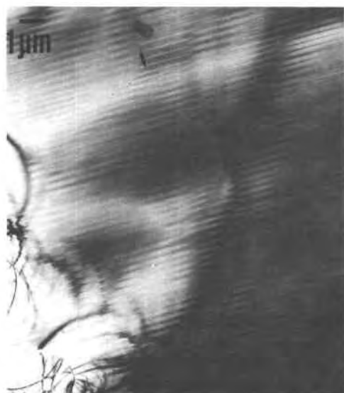
Fig. 1. A TEM image of an ion-thinned foil. Fine layers with period of about 2000 Å are observed throughout the foil.
