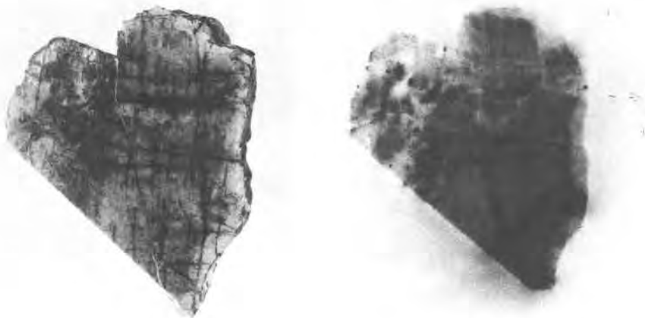
Fig. 2. Cut slab of thalenite from near Kingman, Arizona, natural size. Left: photograph; right: autoradiograph; note the effects of radiation from the sides of the specimen.
