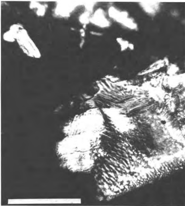
Fig. 6. Harding pegmatite plus 6.0 wt% H 2 O held at 750°C for 168 h. Capsule wall was across top of photomicrograph. Fine dendritic crystals are beta quartz, and the large intergrowth is made up of quartz in an albite lath. Undercoolings of the two phases are beta quartz—137°C and albite—60°C. Scale bar = 0.1 mm; cross-polarized light.
