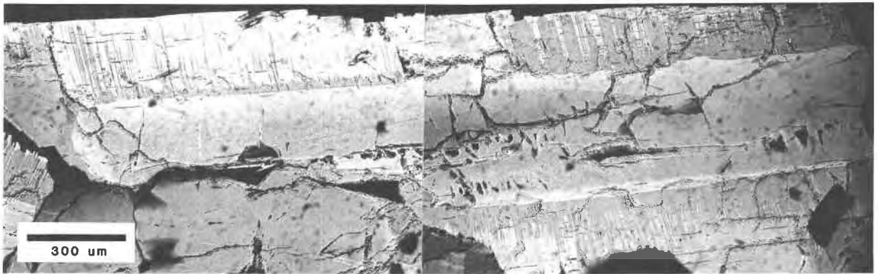
Fig. 1. Lamellar-intergrowth texture along the rim of a normally zoned plagioclase core. The inner, composite zone is dominated by sanidine (dark gray), and the margin, by albitic plagioclase (light gray).
