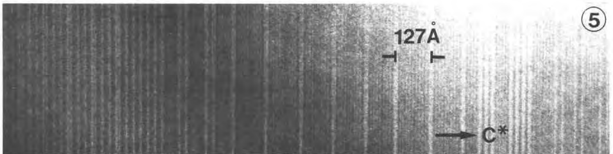
Fig. 3 (upper photograph). An ordered sequence of twinning in leucophoenicite resulting in a superperiodicity with d_{(001)} = 165 \text{ \AA} .
