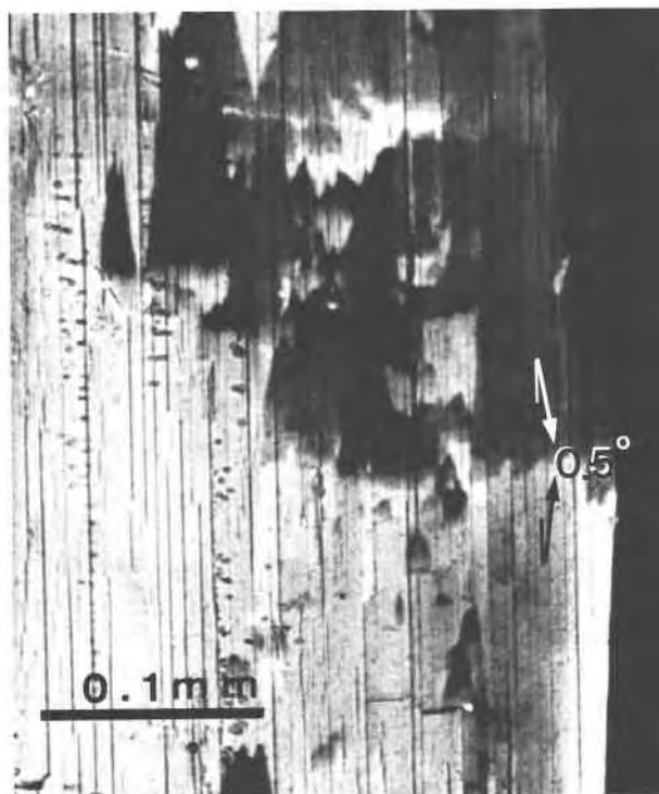
Fig. 4. Polarized photomicrograph showing the {010} sector in the (100) section of brewsterite. The (010) face consists of (0kl) and 0k\bar{l} vicinal faces. Extinction direction and angle from the (010) cleavage plane are indicated. The vertical lines are due to the (010) cleavage. Crossed polars.
