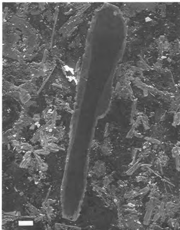
Fig. 5. Mica crystal from mixed mafic phonolite-minette HM-418a (mixed assemblage 4). A rounded xenocrystic core of phlogopite (dark gray) is in sharp contact with a more Fe-Ti-rich mantle. This is surrounded by an outer rim of biotite (light gray), which is similar to biotite in the groundmass. Backscattered-electron image; scale bar is 100 \mu\text{m} .
