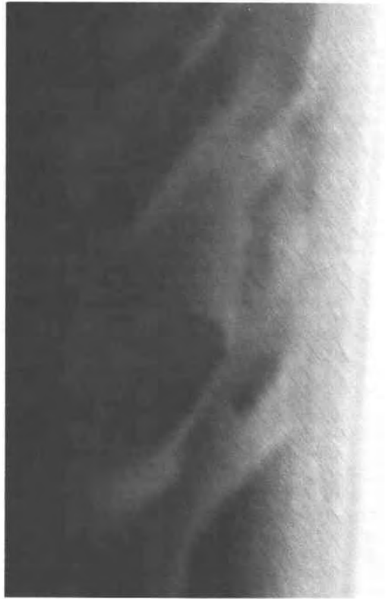
Fig. 5. Microstructure in synthetic Opx, consisting of irregular domains of opposite contrast (rarely observed). Two-beam dark-field image; short dimension = 30 \mu\text{m} ; g = 832 .
