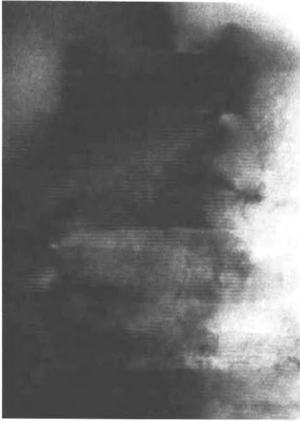
Fig. 4. Typical straight defects parallel to (100) in synthetic Opx. Short dimension of image = 0.15 \mu\text{m} .
