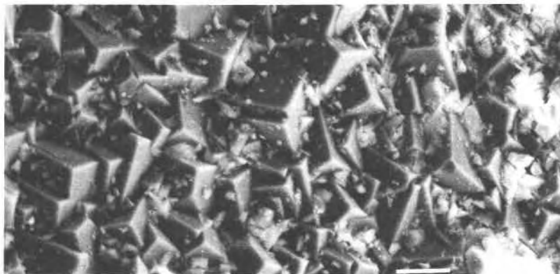
Fig. 1. SEM micrograph of synthetic ammonioalunite with characteristic rhombohedral faces. White bar represents 10 \mu\text{m} .
