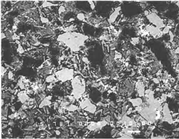
Fig. 1. Backscattered-electron image (scale bar: 10 \mu\text{m} ) of a quenched run product. Lightest-gray grains are grossular, medium-gray needlelike crystals are anorthite, darkest grains are kyanite or quartz. Medium-gray interstitial area is a mixture of aluminosilicate melt and tiny anorthite crystals. Small bright spots are bits of \text{Li}_2\text{MoO}_4 . Photo courtesy of John Laughlin.
