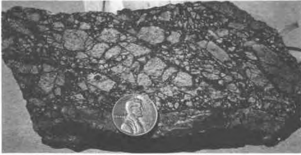
Fig. 9. Photograph of tourmaline- and fluorite-supported breccia, Dysart area. Clasts are composed of silicified and feldspathized Flying W conglomerate. Small quartz vein at base of rock.
