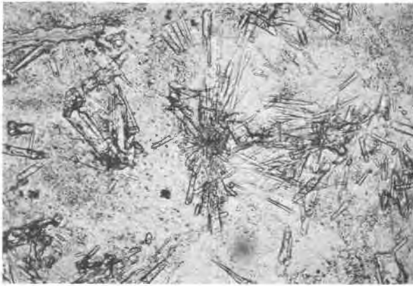
Fig. 6. Photomicrograph of elongate, radiating topaz grains, Dysart dike. Plane-polarized light. Field of view about 700 \mu\text{m} across.
