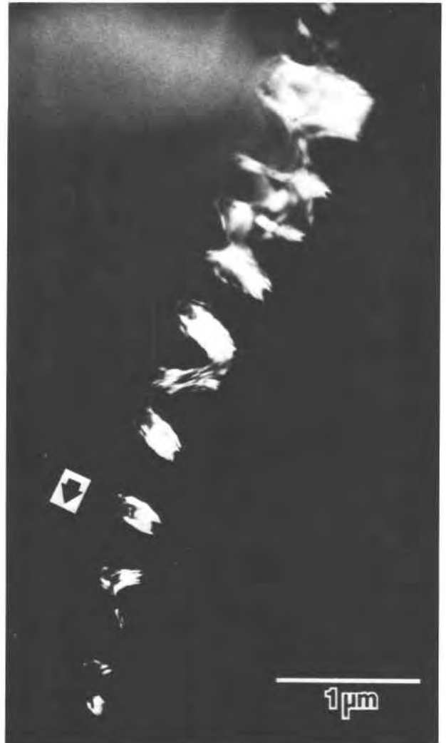
Fig. 13. Helical edge dislocation in anisotropic garnet. The arrow shows the stacking direction of {110} growth layers.
