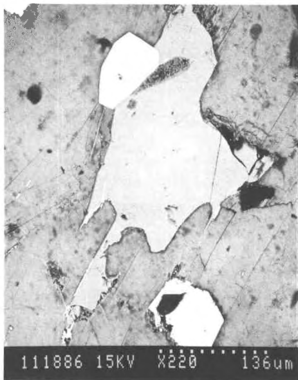
Fig. 2. Backscattered-electron image of a thin section containing defernite (gray), hillebrandite (light gray), and hausmanite (white).
