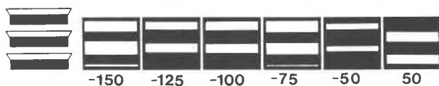
Fig. 2. Simulated 1-D HRTEM images of kaolinite shown as a function of focus conditions (shown beneath each image as deviations from Gaussian focus). Scherzer focus for the Philips 420T is approximately -100 nm. Simulations assumed the structure was oriented with the layers perfectly parallel to the electron beam.
