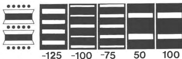
Fig. 4. Simulated 1-D HRTEM images of muscovite. Simulations assumed the structure was oriented with the layers perfectly parallel to the electron beam.
