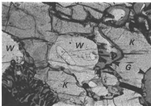
Fig. 2. Kornerupine (K) enclosing werdingite (W) that contains sillimanite inclusions. Replacement of werdingite by grandidierite (G) ( \pm hercynite) occurs at kornerupine-werdingite boundaries. In the bottom left corner, grandidierite-hercynite symplectite replaces werdingite from a hercynite-werdingite boundary. Photo length is 2 mm.
