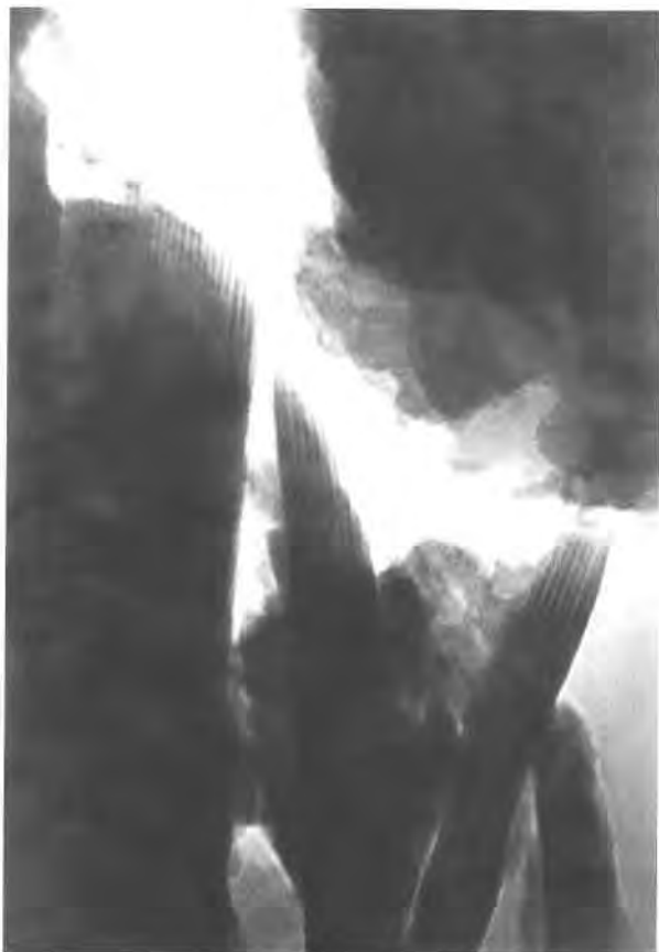
Fig. 1. Lattice fringe image obtained using 00l reflections. Fringes have d = 36 \text{ \AA} , with weak subfringes.
