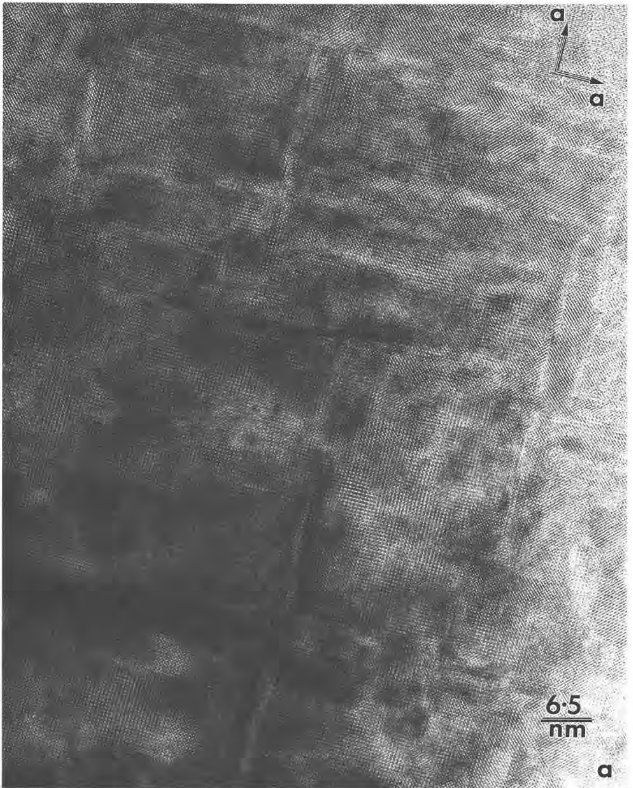
Fig. 2. (a) High-resolution images viewed down [001] of rutile (sample 2113) illustrating the presence of platelets parallel to (100) and (010) of rutile.
