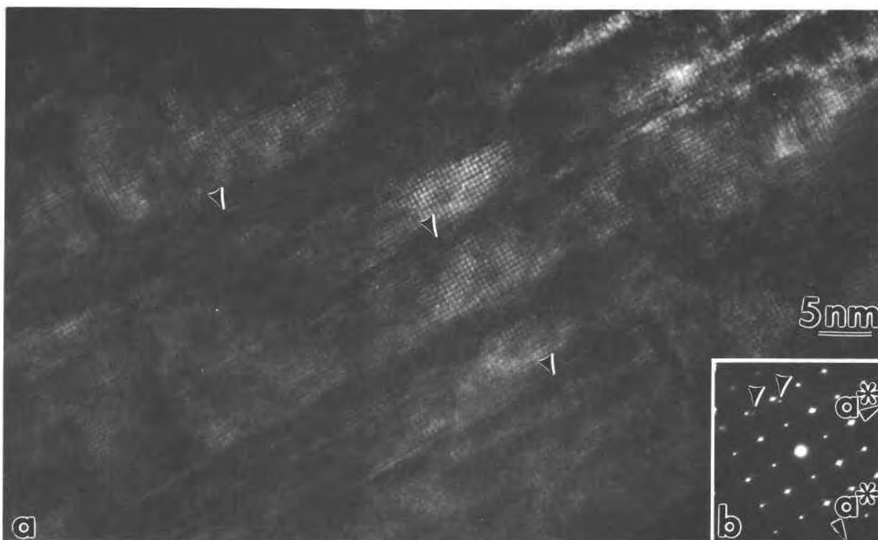
Fig. 9. (a) The [001] zone of rutile (sample 18) showing unequal development of lamellae (arrowed) parallel to (010) and (100) of rutile; (b) SAED pattern for a illustrating a slight rotation of the lattice of the lamellae (arrowed) relative to that of the rutile.
