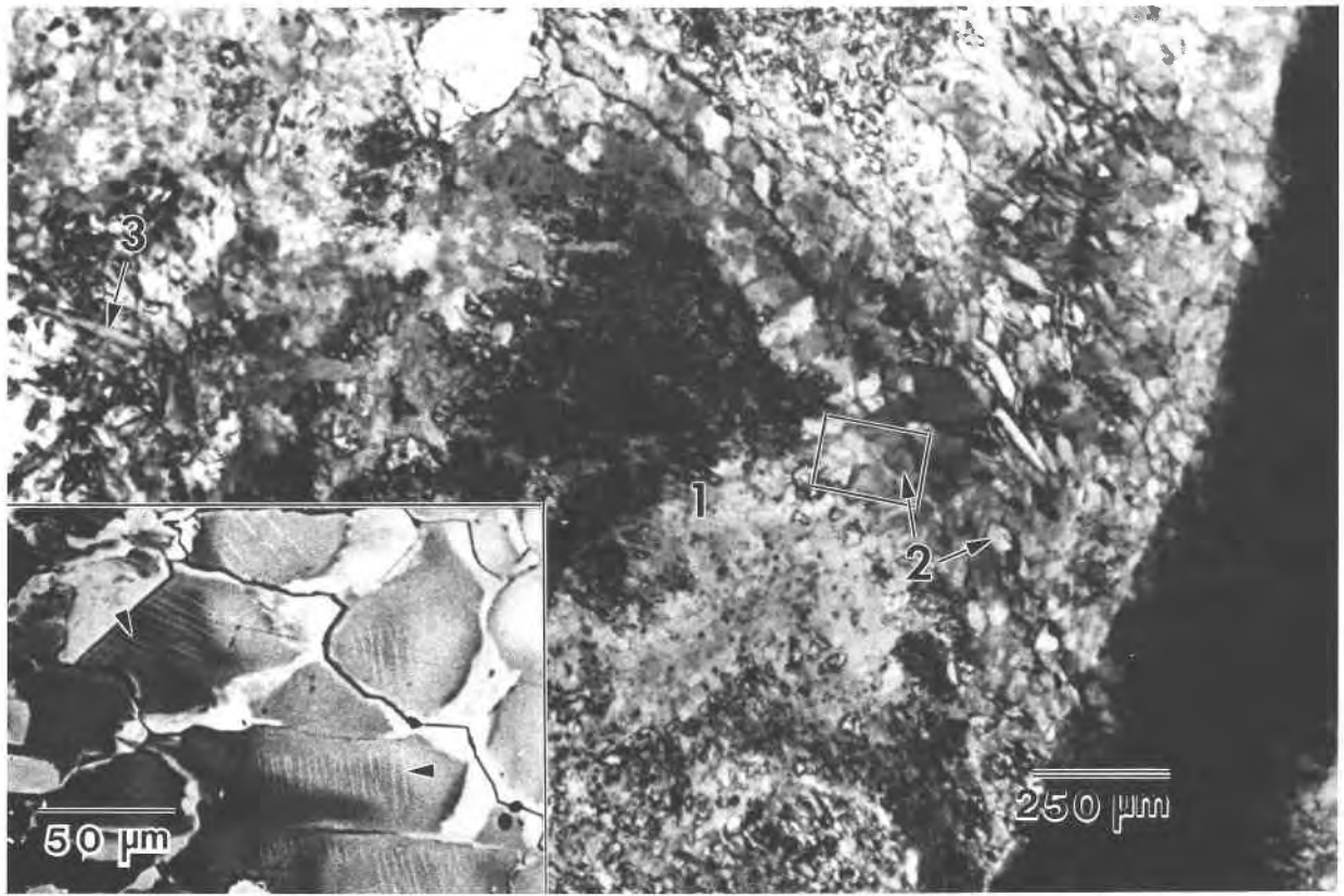
Fig. 1. Plane polarized light micrograph of complex amphibole assemblage in the least deformed amphibolite boudin. The amphiboles occur as large, inclusion-filled porphyroclasts (1), equant subgrains (2), and postkinematic needles (3). The inset shows a higher magnification backscattered electron image of the subgrains (boxed area) containing narrow "100" and "101" cummingtonite lamellae (arrows). The porphyroclasts and subgrains were found to contain pervasive actinolite-hornblende exsolution.
