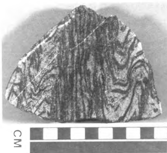
Fig. 1. Photograph of Mn-rich assemblage from Arnold pit. Black layers are dominantly braunite; light layers are dominantly Mn-rich calciferous amphibole.
