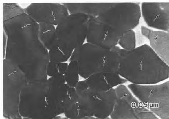
Fig. 2. Low-magnification image of crocidolite along [001], showing the cross sections of fibrous crystals. Many cross sections are irregular in outline. The arrows indicate the a^* direction, which was determined from the orientation of intergrown wide-chain slabs.
