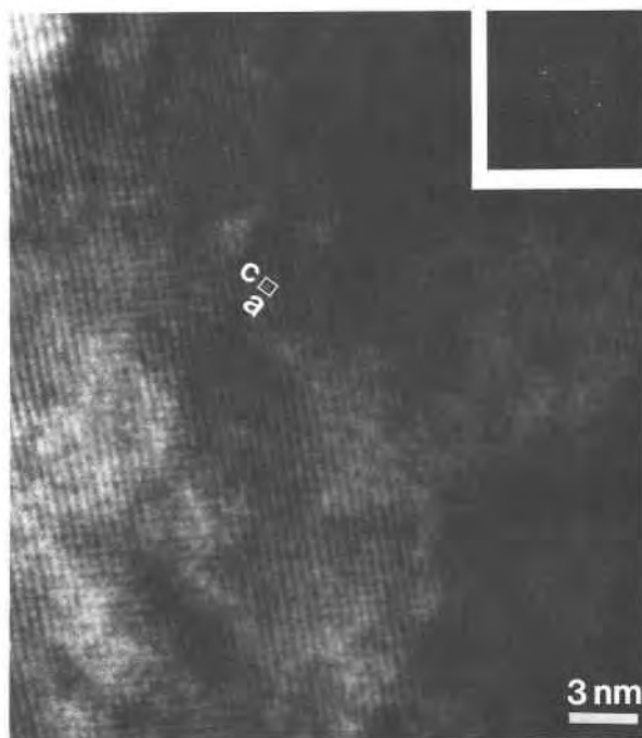
Fig. 12. Two-dimensional lattice image in the (010) plane and electron diffraction pattern. Lattice-fringe distortion and discontinuities become more apparent. Aperiodic domains increase in number and begin to overlap.
