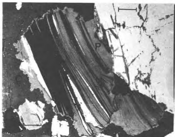
Fig. 1. Backscattered electron image of pumpellyite (P) intercleaved with phlogopite (black) between braunite (white) and calcite (C) in Assemblage 2. Note veins of pumpellyite in braunite. Length of the bar is 0.01 cm.
