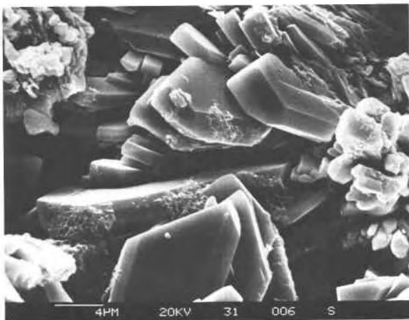
Fig. 2. Secondary electron image of synthetic iron lithium staurolite \text{Fe}_3\text{Li}_1\text{Al}_{18.33}\text{Si}_{7.5}\text{O}_{48}\text{H}_4 . Bar scale is 4 \mu\text{m} .
