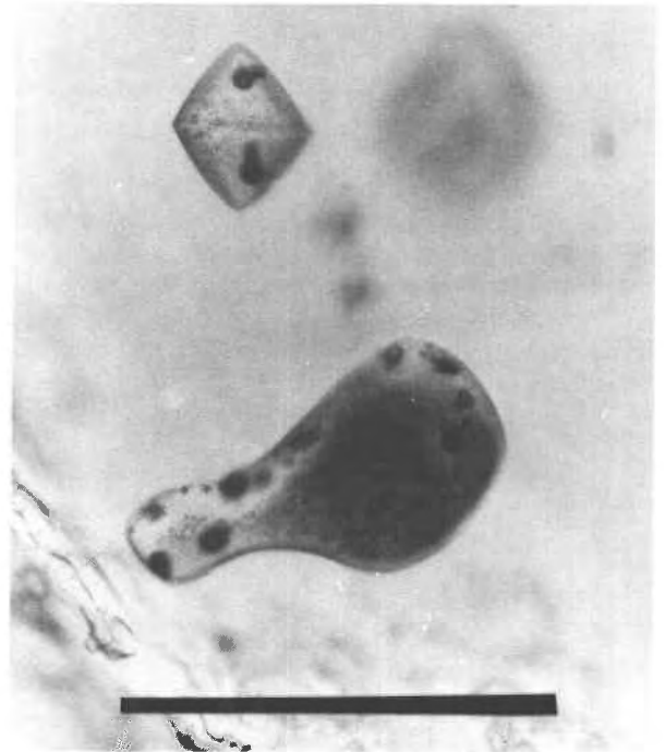
Fig. 15. Round and faceted inclusions in a Mono quartz. The larger, rounder inclusion extends to a position closer to the glass-coated rim of the quartz. The scale bar is 200 \mu\text{m} long.
