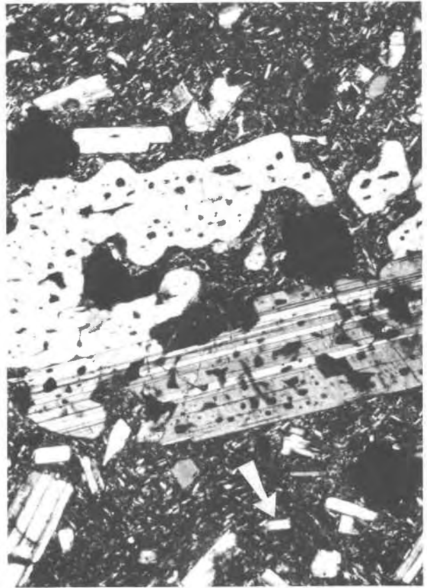
Fig. 1. Photomicrograph of the starting material containing large resorbed plagioclase phenocrysts typical of many intermediate and mafic lavas. Arrow indicates a member of a second population of euhedral, often more calcic, plagioclase microphenocrysts.
