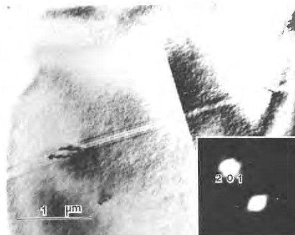
Fig. 16. Dark-field image of a \frac{1}{2}[100] stacking fault with symmetrical fringes and dislocations in perovskite from Akhmatov. Two-beam condition with 201 operating.
