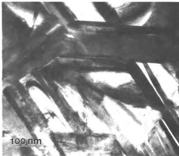
Fig. 17. Aggregate of anatase needles with a high intercrystal porosity.
