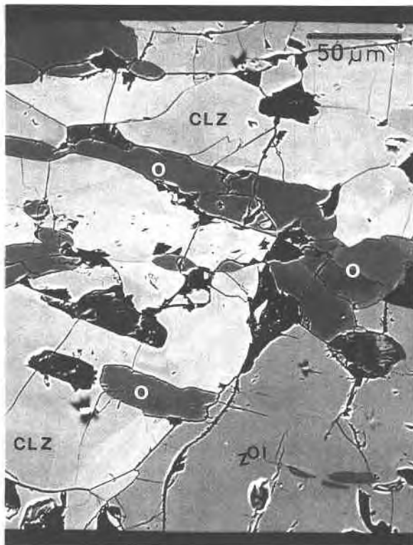
Fig. 9. Backscattered electron image of clinozoisite and zoisite from eclogites equilibrated at 2 GPa (sample DT-8), together with omphacite (O) and amphibole (black, not labeled). The omphacite crystal in the lower left grows across the grain boundary between zoisite and clinozoisite and also across the core (Fe poor, 37 mol% \text{Al}_2\text{Fe} ) and the rim (Fe rich, 49 mol% \text{Al}_2\text{Fe} ).
