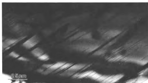
Fig. 4. An area of an olivine crystal containing abundant dislocations that are decorated by layers parallel to (001) olivine.
