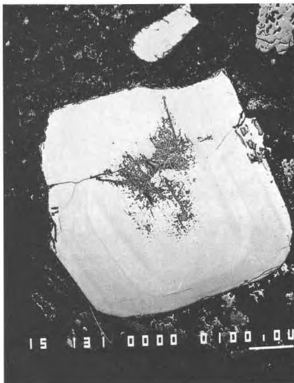
Fig. 6. BSE image of a partially altered plagioclase phenocryst from sample 212J. Scale bar is 100 \mu m. The core of the plagioclase has been extensively altered, and replacement has taken place by the development of a vermicular texture, with abundant narrow tubes. Locally, where cracks extend to the rim, alteration is more extensive, indicating that the cracks acted as pathways for infiltrating fluids.
