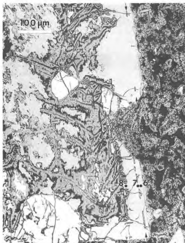
Fig. 2. BSE image of a partially altered plagioclase (light gray) from 212L, in which the calcic core has been replaced by amorphous \text{SiO}_2 (dark gray). Oscillatory zoning is present in this feldspar, which ranges from An_{64} at the rim to An_{70} at the edge of the altered core. Incipient alteration can be observed along a calcic zone (arrows) of An_{70}\text{--}An_{73} that has been partially replaced within the relict plagioclase. Numbers correspond to analyses in Table 1.
