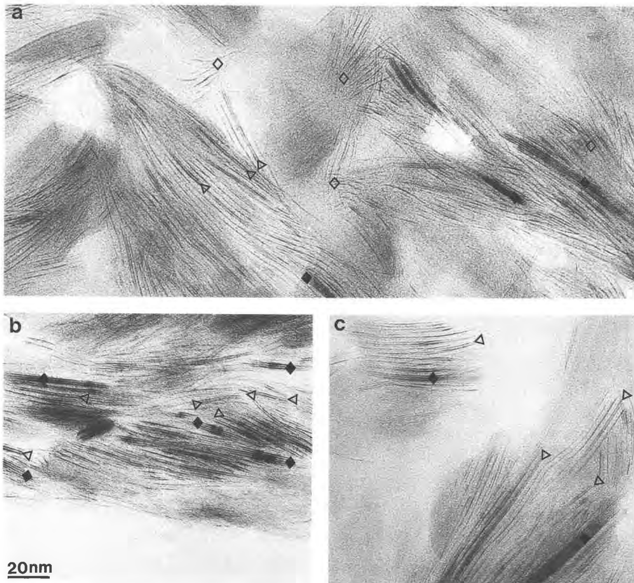
Fig. 5. (a–c) TEM images of aggregates in one octadecylammonium-treated ultrathin section of the original (i.e., without pre-treatment) sample (509B-2-1, 44–48 cm) from the Galapagos Spreading Center, showing different types of layer structures. In general, the morphological features are similar to those illustrated in Fig. 4, except that the open diamonds refer to layers of nontronite in nonparallel stacking and random spacing (13–30 Å). The nonexpandable component consists of celadonite or glauconite (Buatier et al., 1989). Symbols in b and c have the same significance as in Fig. 4. Scale bar is the same in all three photos.
