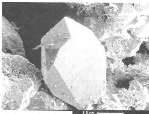
Fig. 1. SEM photograph of a synthetic ammonium feldspar crystal grown at 600 °C and 2 kbar. Flaky material on both sides of the crystal is carbon substrate material.
