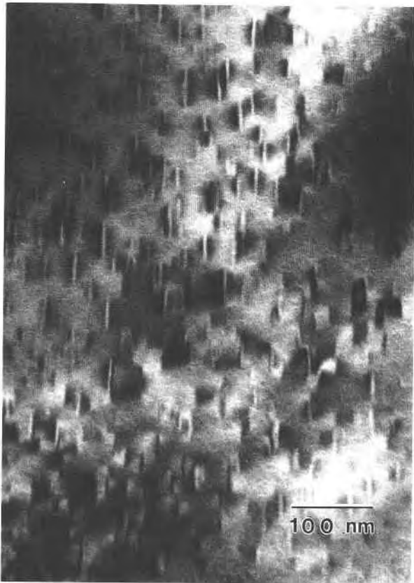
Fig. 3. Bright-field TEM image showing homogeneously distributed Guinier Preston (GP) zones of gedrite in anthophyllite host. These tiny platelets are parallel to (010) and were common in most samples. The beam is near [001]. Microstructure from sample 89-18B.
