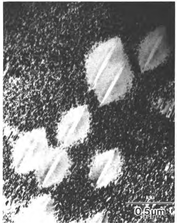
Fig. 14. Bright-field TEM image showing evidence for two types of exsolution lamellae in gedrite. The first is represented by the medium-sized disk-shaped lamellae. With additional cooling, there was rapid homogeneous nucleation of abundant GP zones in the solute-enriched areas between the bigger lamellae. Note the distinctive football-shaped solute depletion zones around the larger lamellae. Versions of this texture were common in many of the samples. Beam is near [001]. Microstructure from sample 89-32.
